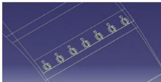
图12 连续光滑后缘变弯结构和喷流控制器的一体化设计 [32] Fig. 12 Integrated design of continuous smooth trailing edge bending structure and jet flow controller [32]
